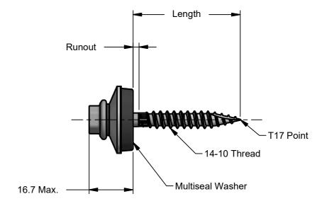
**Note**Lengths from underside of sealing washer and includes compression.
