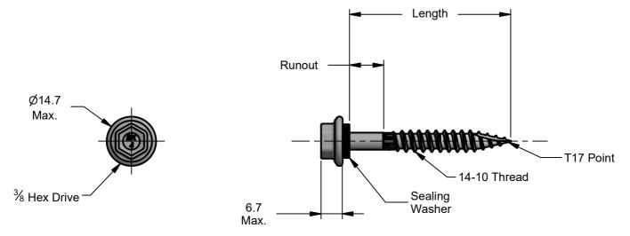
**Note**Lengths from underside of sealing washer and includes compression.
